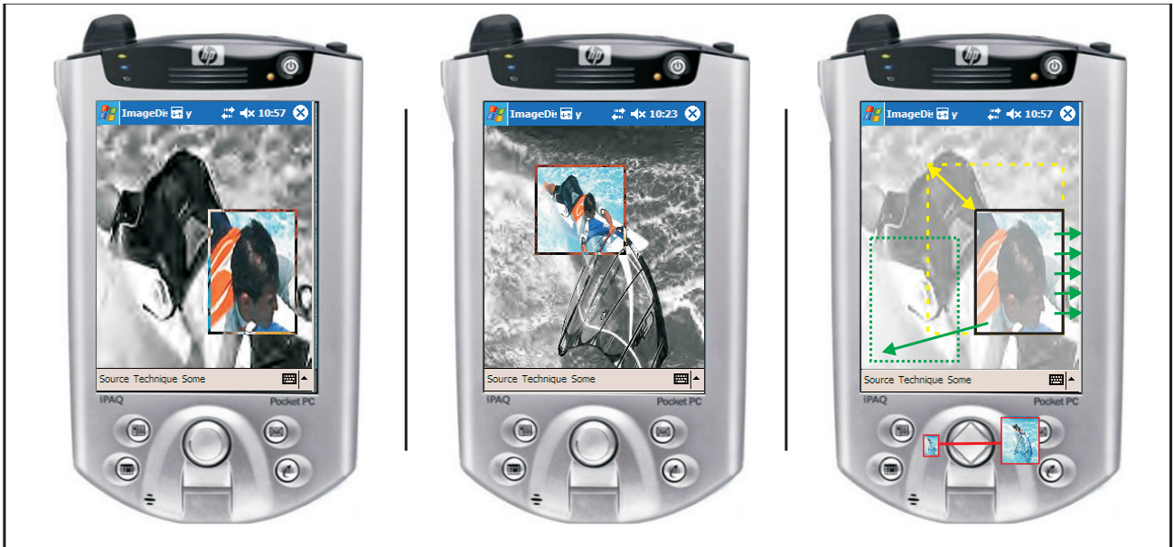
Figure 3. The user interface of the proposed image browsing system: In close-ups, the fully-detailed focus allows for an exploration of currently important image content, whereby the blurred representation of the background provides spatially-undistorted context (left). In overviews, the blurring effect is inherently reduced allowing for better orientation and navigation (middle). The means for interaction involve common elements of modern mobile hardware and support typical browsing interactions (right) as panning focus and background (green), focus resize (yellow), and animated zooming (red).
