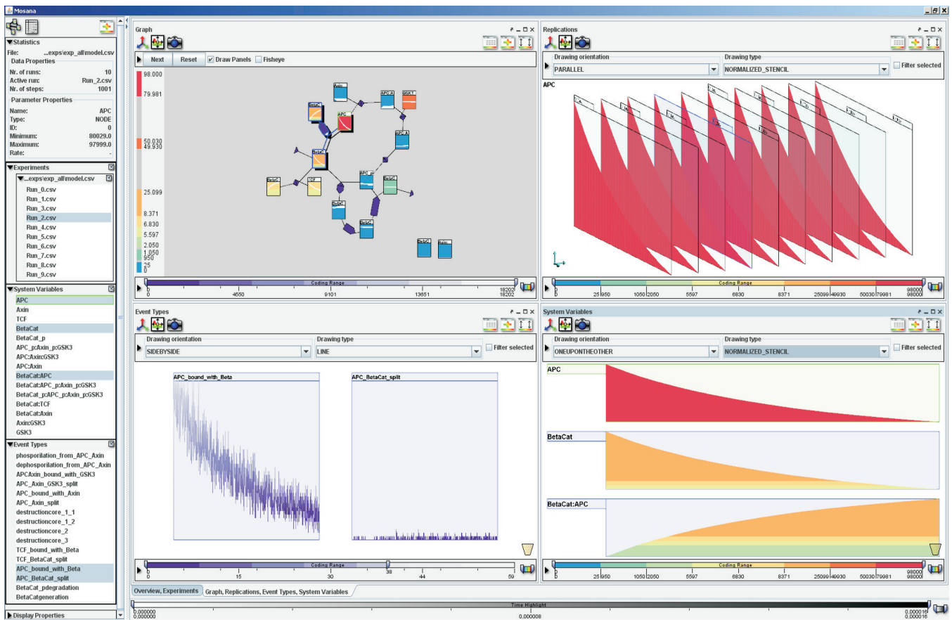
Figure 7: Visualization design for the detailed exploration of one experiment. The Experiment View (top left) is coordinated with the Multi-Run View (top right) for the selection of one run from all runs, the Node View (bottom left) for the detailed analysis of single-run data linked to nodes, and the Edge View (bottom right) that shows the single-run data connected to edges. The data of the icons highlighted by a shadow are shown in the Node and Edge Views. The icon highlighted by green borders is the node shown in the Multi-Run View.
